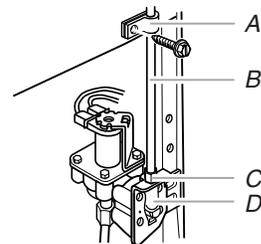
6. The ice maker is equipped with a built-in water strainer. If your water conditions require a second water strainer, install it in the ¼" (6.35 mm) water line at either tube connection. Obtain a water strainer from your nearest appliance dealer.
