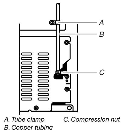
5. Turn shutoff valve ON. Check for leaks. Tighten any connections (including connections at the valve) or nuts that leak.
