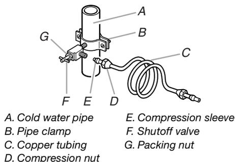
6. Fasten the shutoff valve to the cold water pipe with the pipe clamp. Be sure the outlet end is solidly in the ¼" drilled hole in the water pipe and that the washer is under the pipe clamp. Tighten the packing nut. Tighten the pipe clamp screws slowly and evenly so washer makes a watertight seal. Do not overtighten or you may crush the copper tubing.
